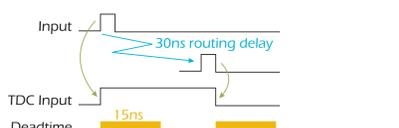
The falling edge of the input can not be detected due to the intrinsic dead-time of the TDC. Instead, routing is used to delay the falling edge until the TDC is ready again.
